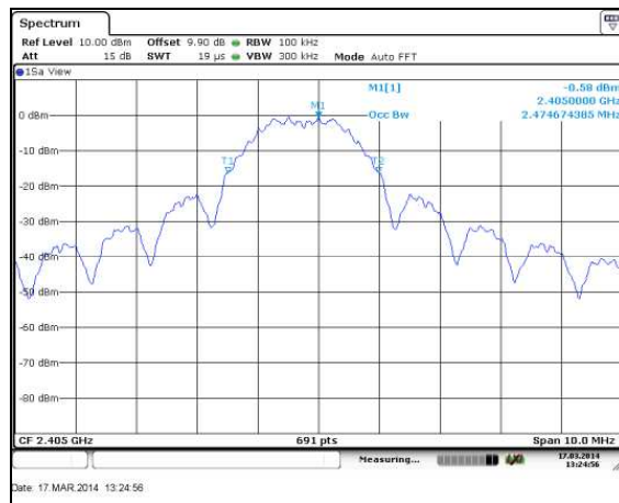
Figure 7.3.2-4: 99% Bandwidth Plot – 2405 MHz
