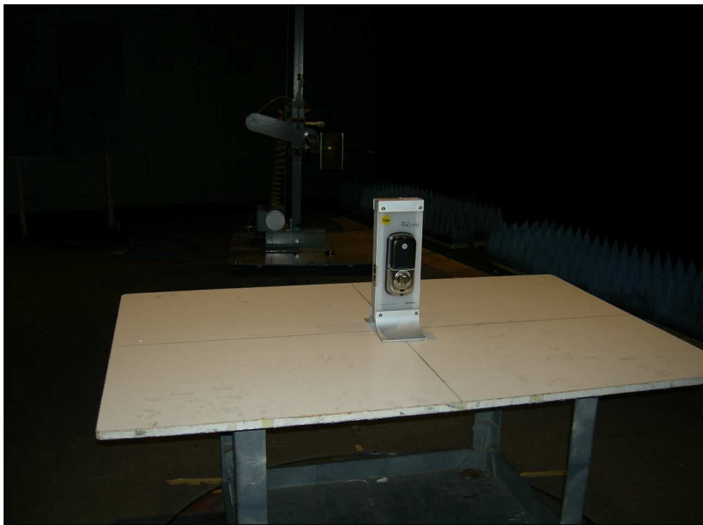
Figure 6: Radiated Emissions – Key Free Touchscreen Deadbolt – YRD240
