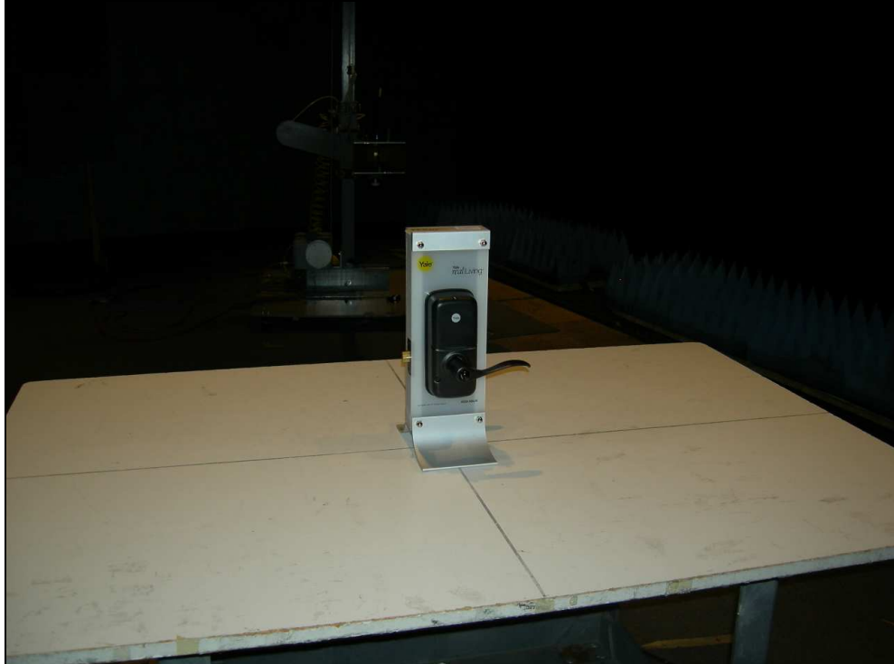
Figure 10: Radiated Emissions – Push Button Lever – YRT210
