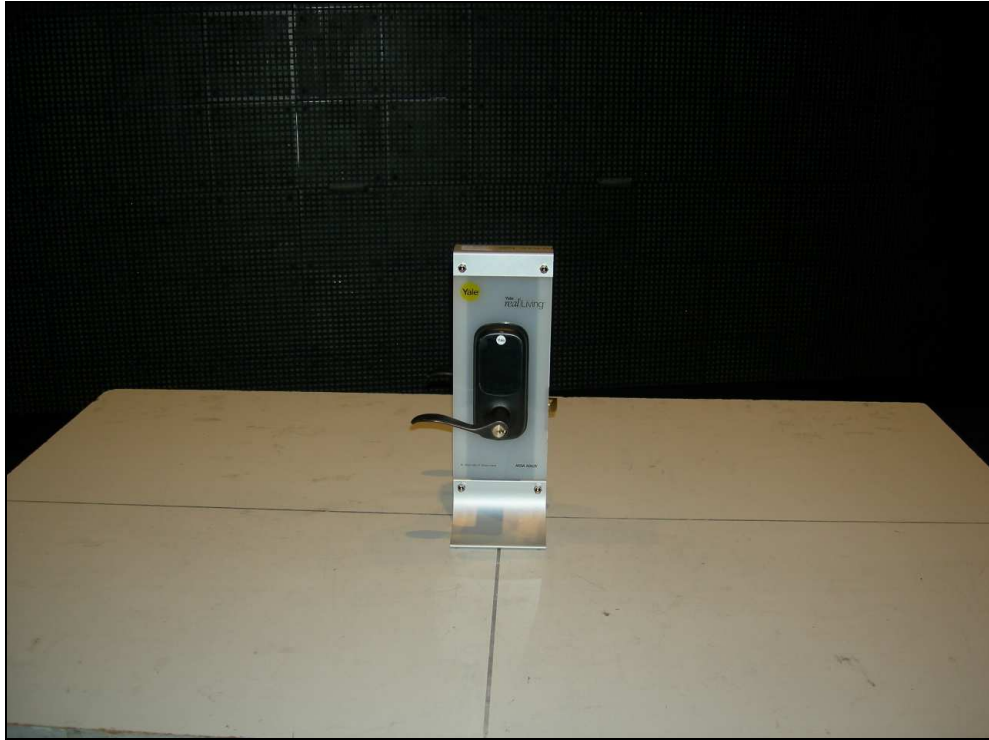
Figure 7: Radiated Emissions – Touchscreen Lever – YRT220
