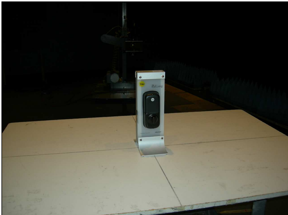
Figure 4: Radiated Emissions – Push Button Deadbolt – YRD210
