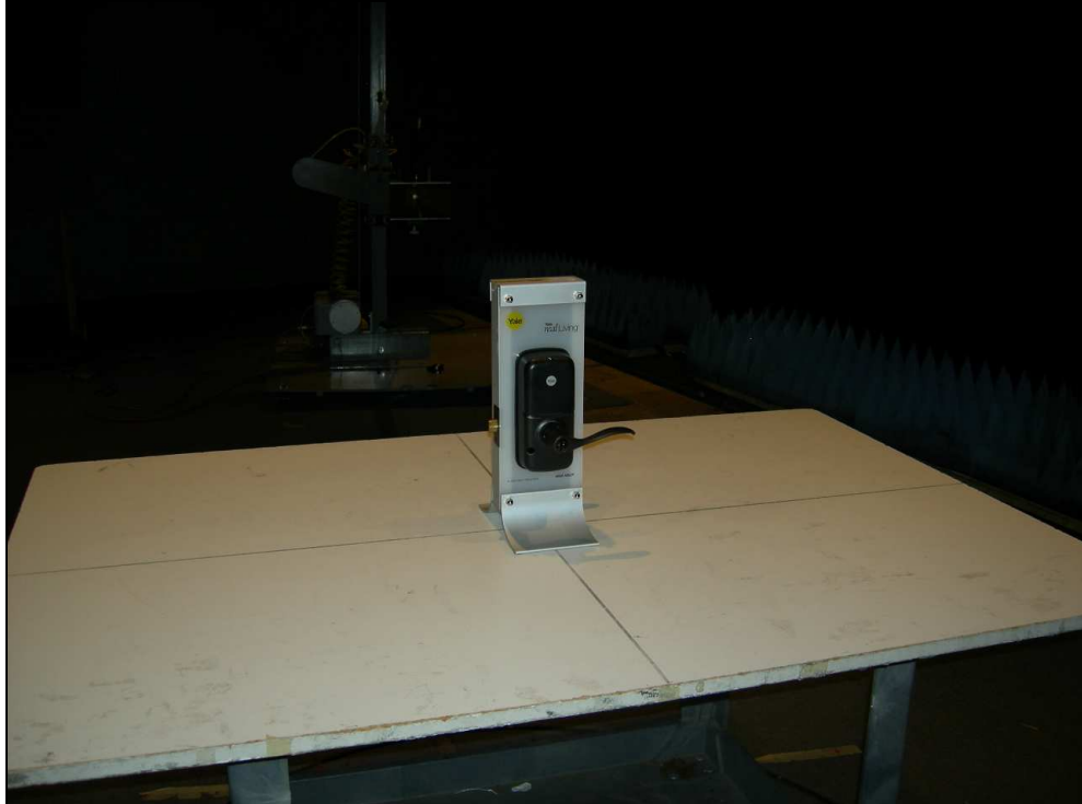
Figure 8: Radiated Emissions – Touchscreen Lever – YRT220
