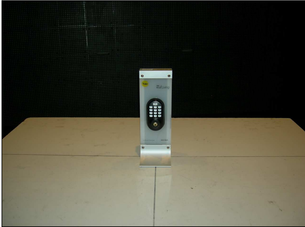
Figure 3: Radiated Emissions – Push Button Deadbolt – YRD210
