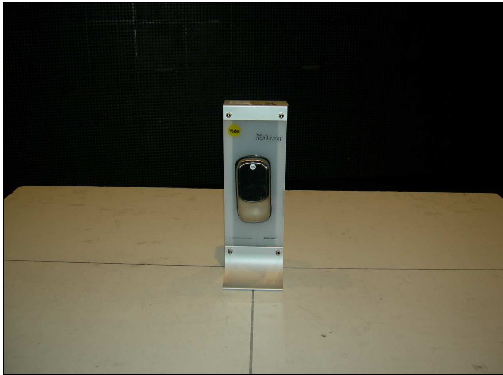
Figure 5: Radiated Emissions – Key Free Touchscreen Deadbolt – YRD240
