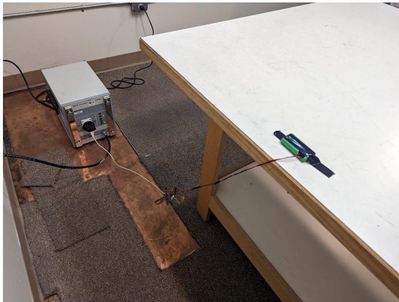
Photograph 6: Back View Conducted Emissions Worst-Case Configuration
