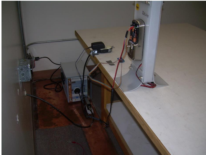
Photograph 6 – Back View Conducted Emissions Worst-Case Configuration
