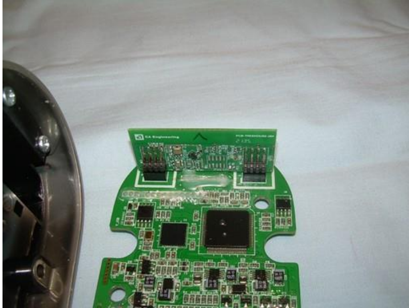
Photograph 1 – Radio PCB Mounted to Main PCB
