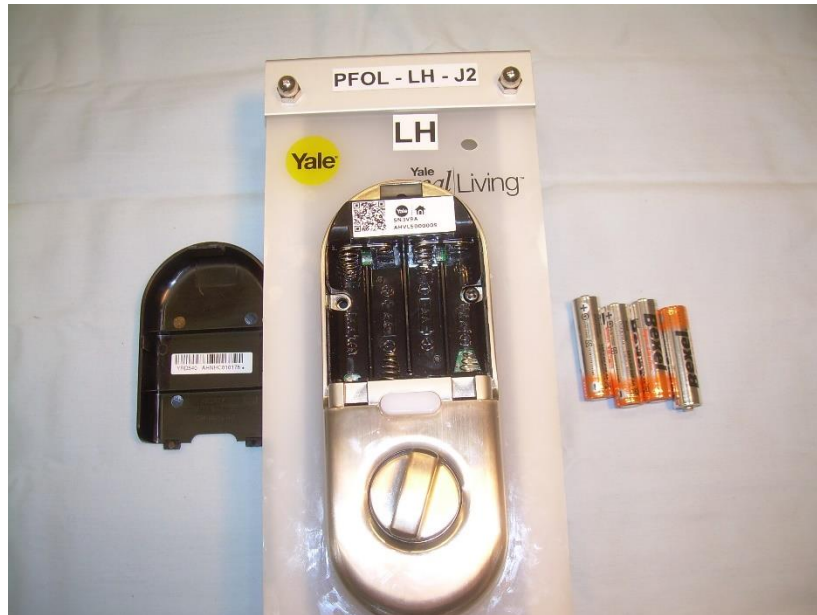
Photograph 7: View of the EUT with Battery Cover Removed
