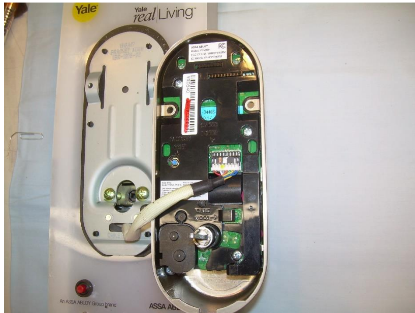
Photograph 8: PCBs Installed in the Lock
