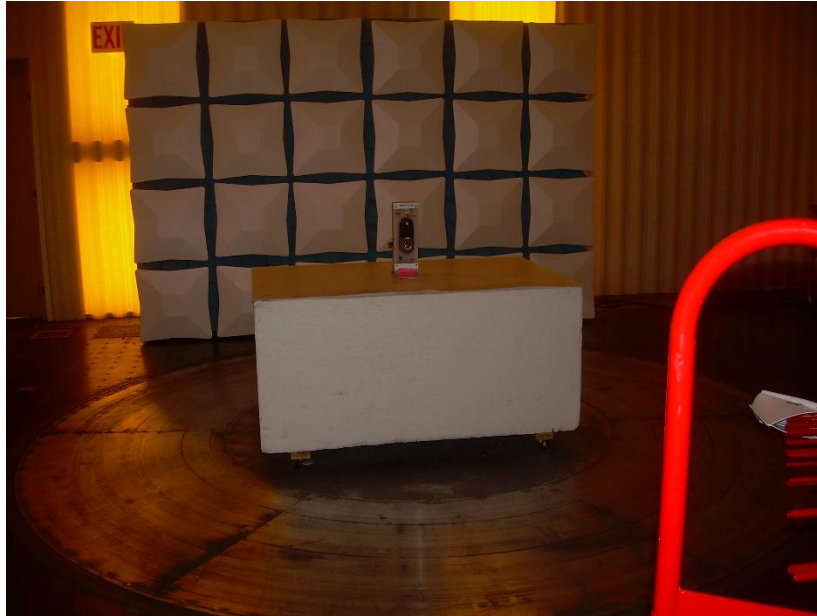
Photograph 1: Front View Radiated Emissions Configuration – 30 to 1000 MHz
