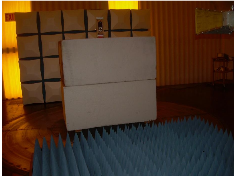
Photograph 3: Front View Radiated Emissions Configuration – Above 1000 MHz
