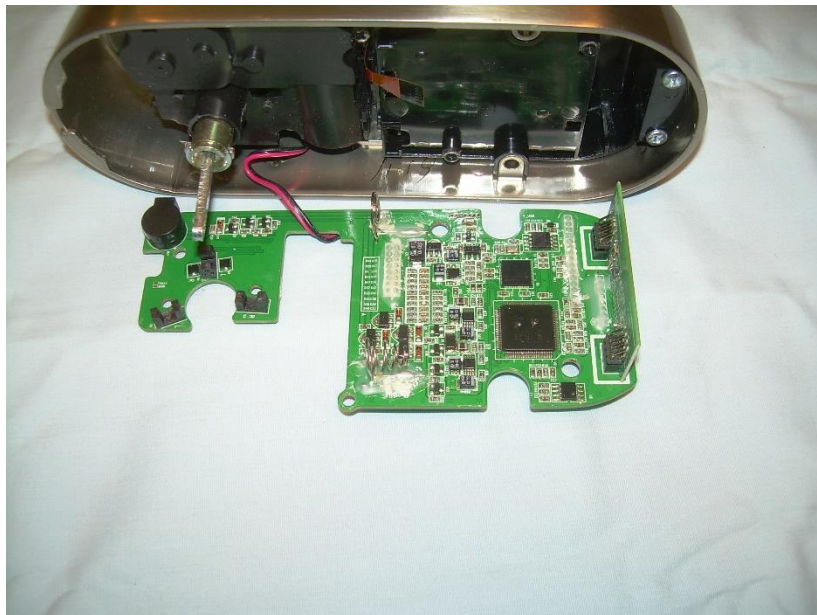
Photograph 10: View of the Front Side of the Main PCB with Transceiver PCB Connected
