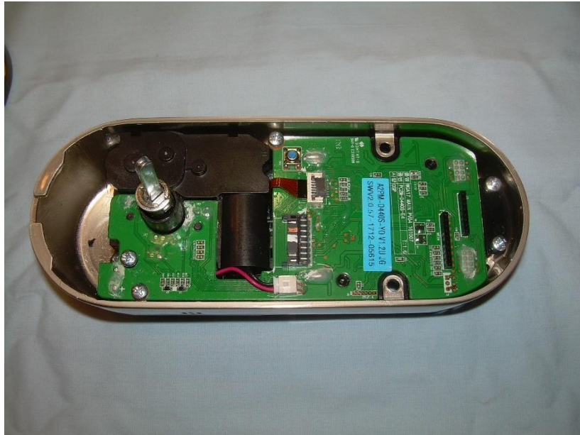
Photograph 9: View of the Back Side of the Main PCB in Housing
