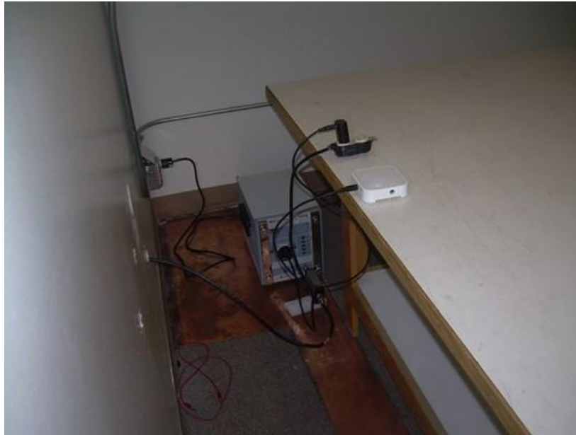
Photograph 5: Back View Conducted Emissions Worst-Case Configuration
