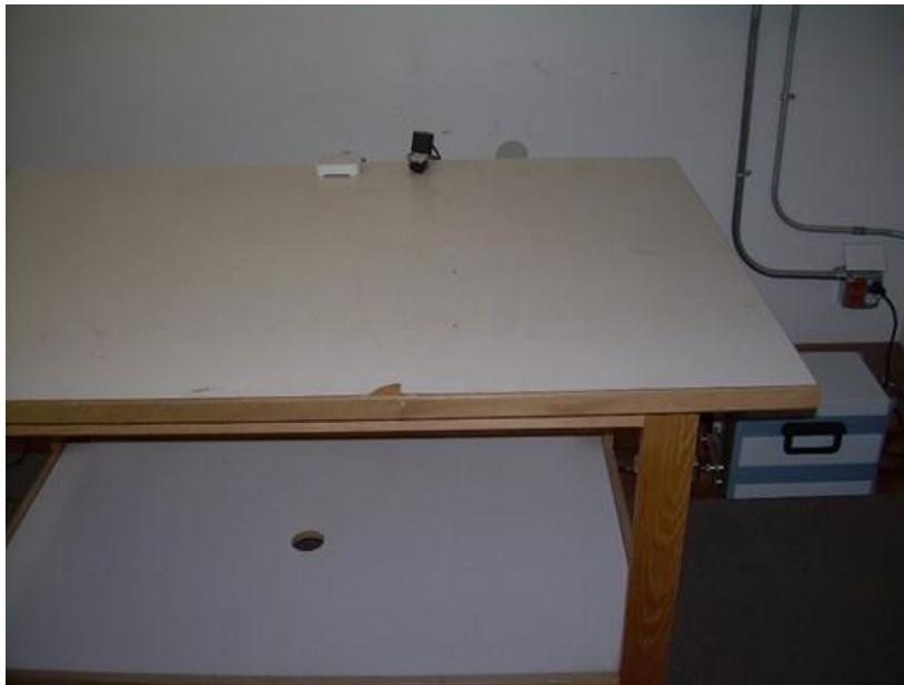
Photograph 4: Front View Conducted Emissions Worst-Case Configuration
