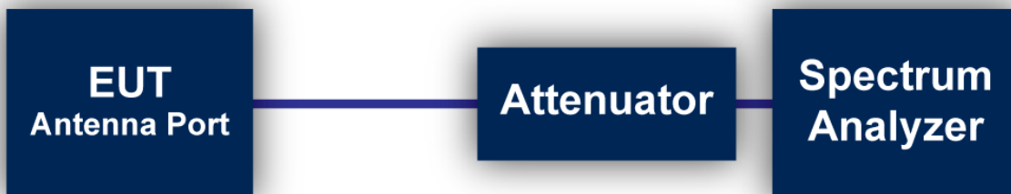
Figure 2: Direct Connection at the Antenna Port Test
