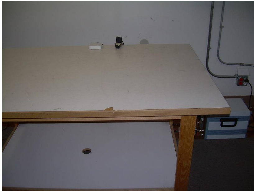
Photograph 4: Front View Conducted Emissions Worst-Case Configuration
