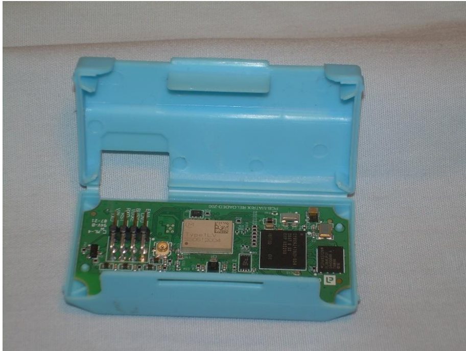
Photograph 7 – PCB Mounting in Housing View
