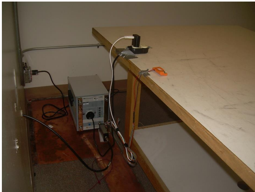
Photograph 8: Back View Conducted Emissions Worst-Case Configuration
