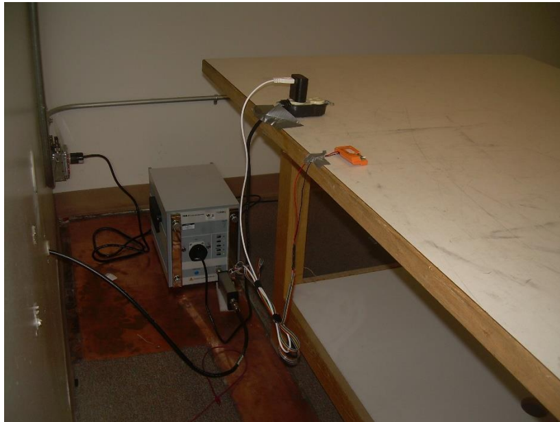
Photograph 8: Back View Conducted Emissions Worst Case Configuration
