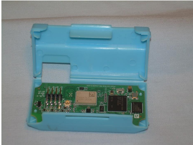
Photograph 15: PCB in Housing
