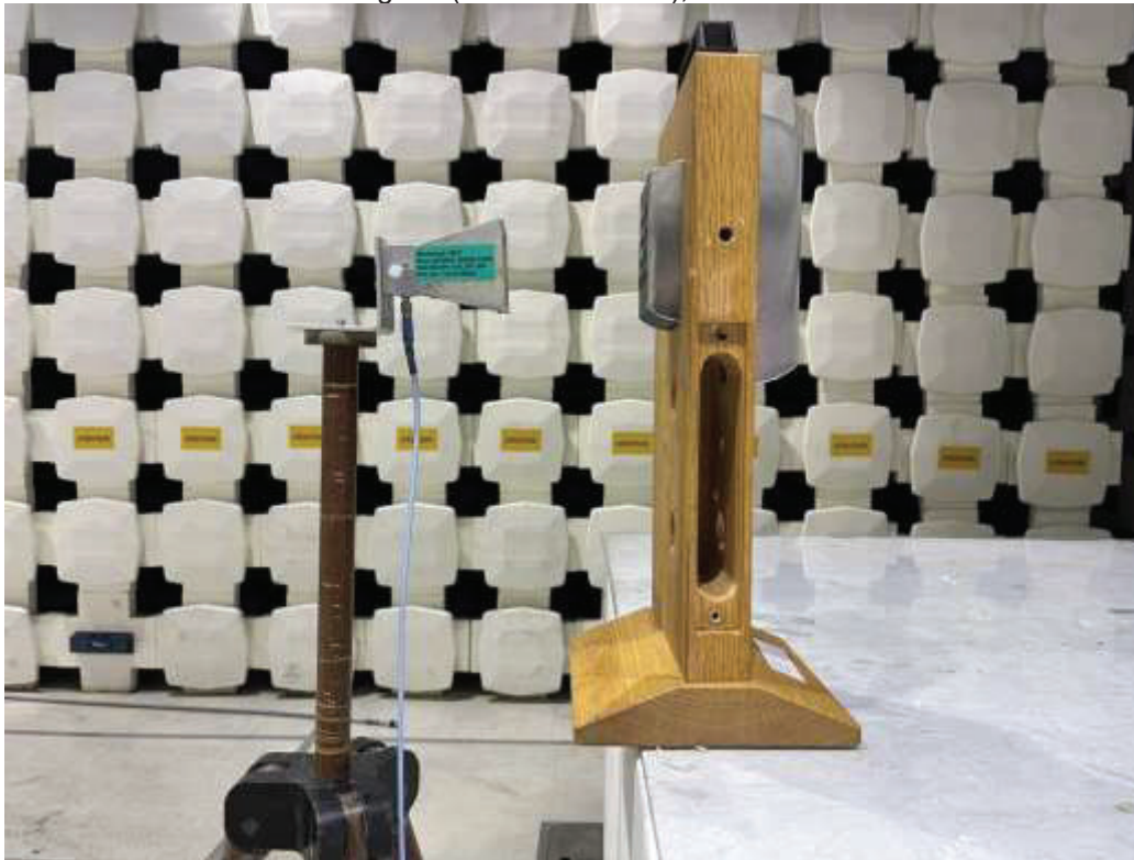
BLE & Zigbee (Metal Enclosure), RE 18-25 GHz
