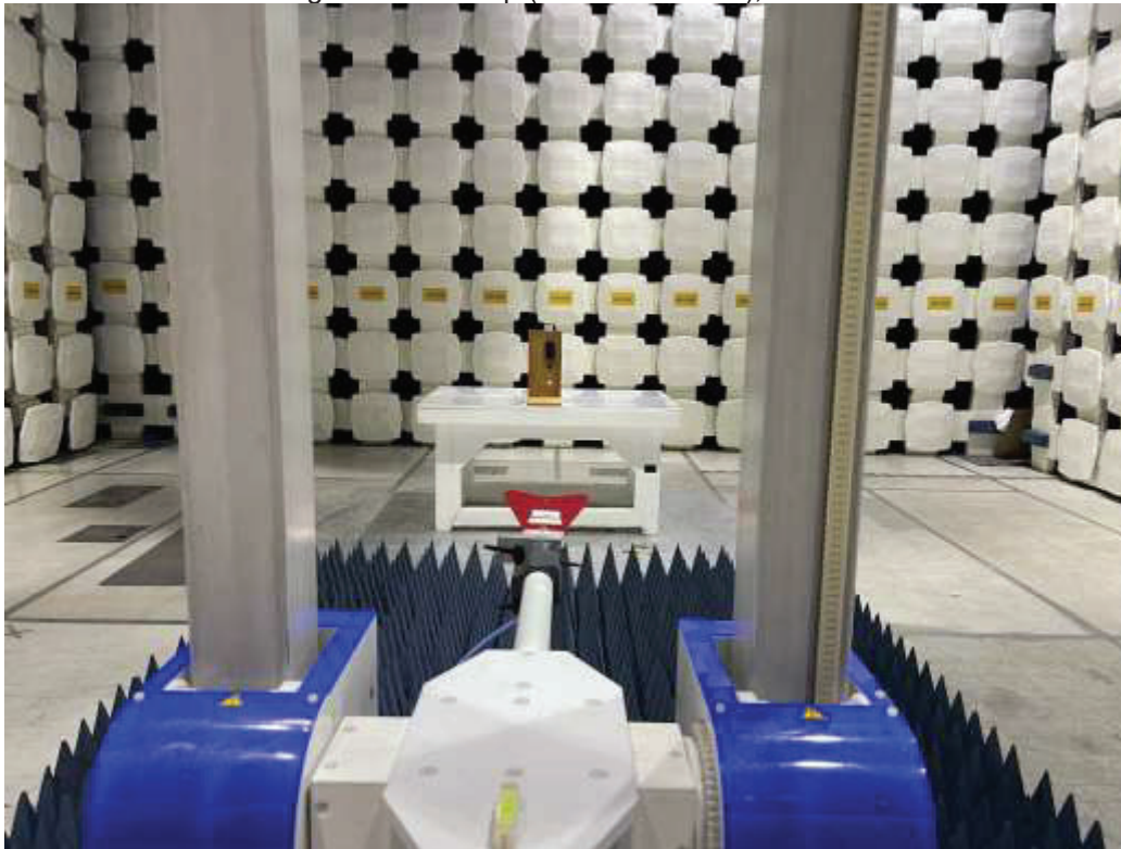
BLE & Zigbee Test Setup (Metal Enclosure), RE 1-13 GHz
