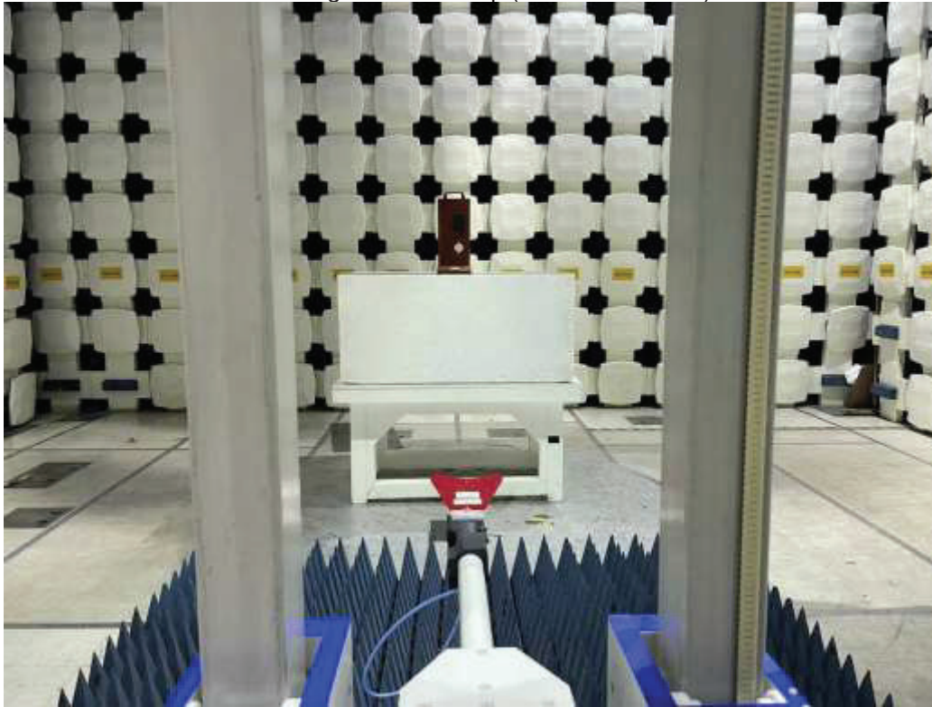
BLE & Zigbee Test Setup (Plastic Enclosure)
