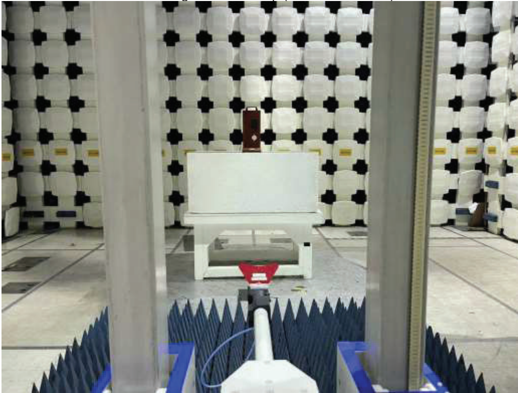
BLE & Zigbee Test Setup (Plastic Enclosure)
