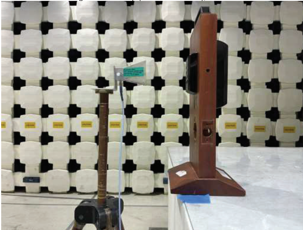
BLE & Zigbee Test Setup (Plastic Enclosure), RE 18-25 GHz
