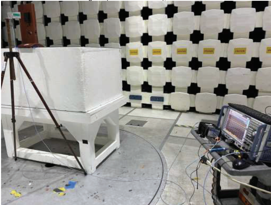
BLE & Zigbee (Plastic Enclosure), RE 18-25 GHz
