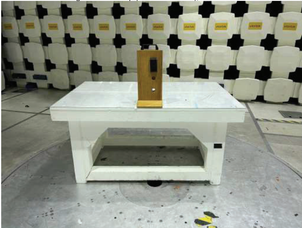
BLE & Zigbee Test Setup (Metal Enclosure), RE 30-1000 MHz
