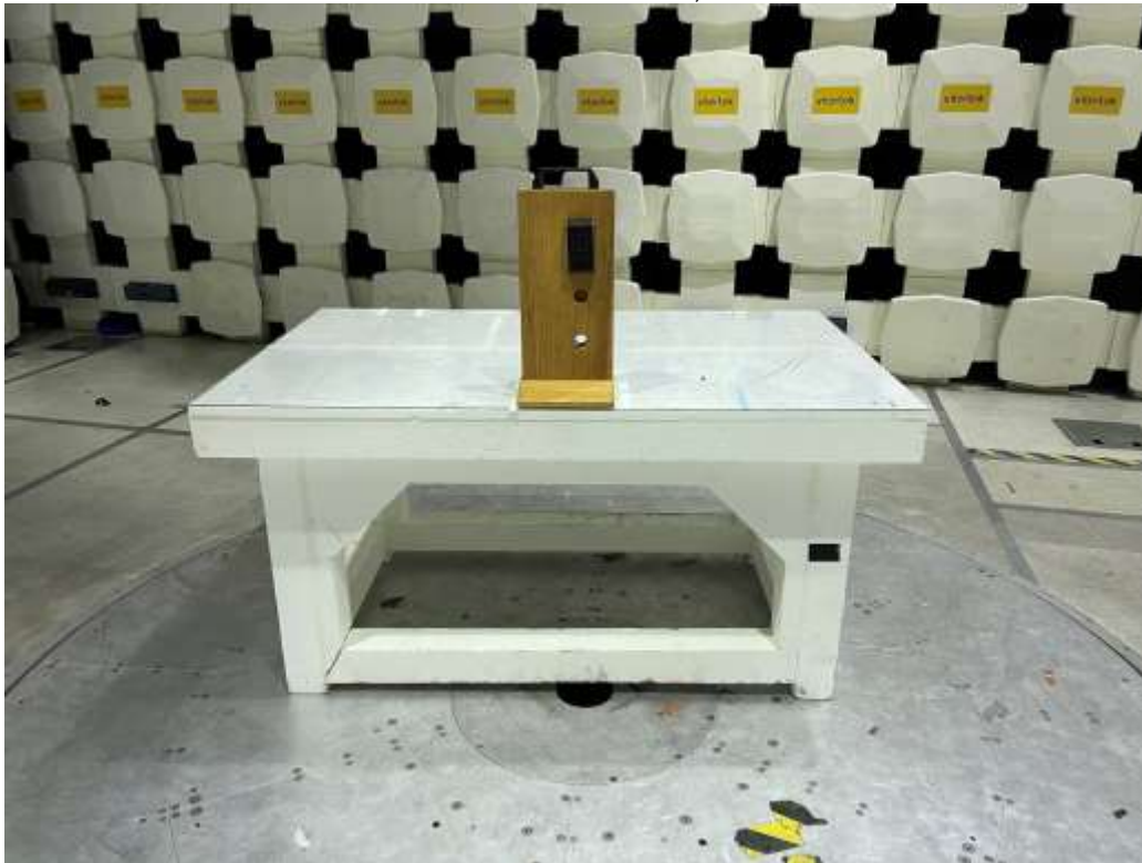
125 kHz RFID With Metal Enclosure, RE 30-1000 MHz
