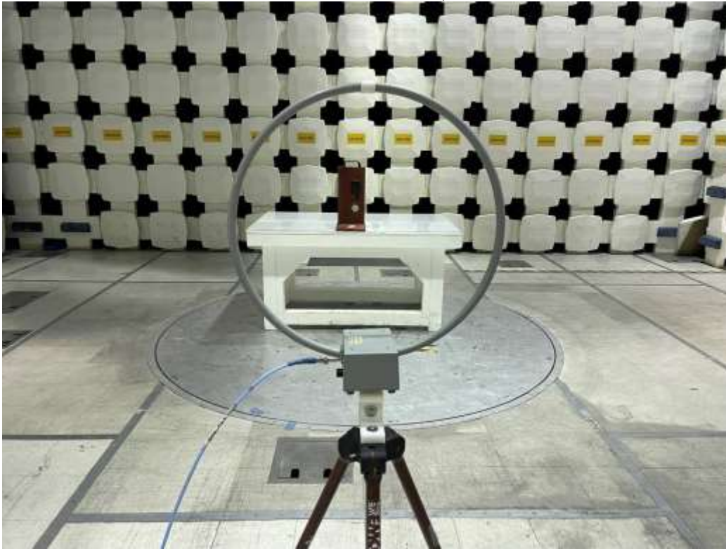
125 kHz RFID With Plastic Enclosure, RE 9 kHz-30 MHz
