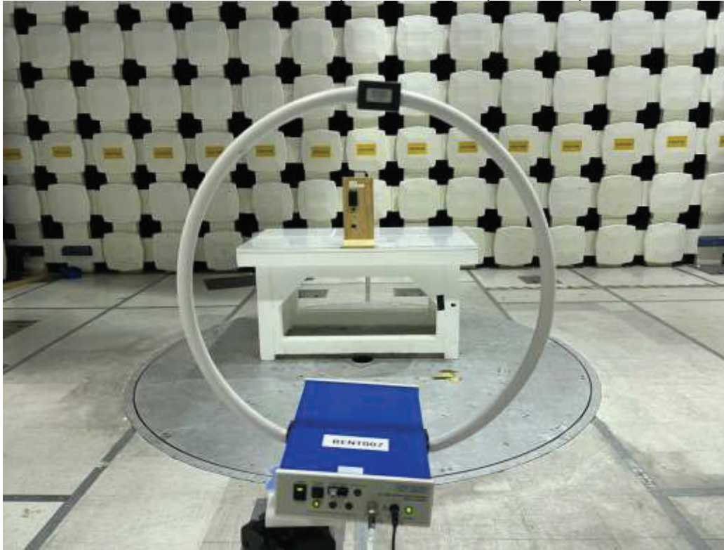
125 kHz and 13.56 MHz RFID (Plastic Enclosure) Test Setup, X-axis
