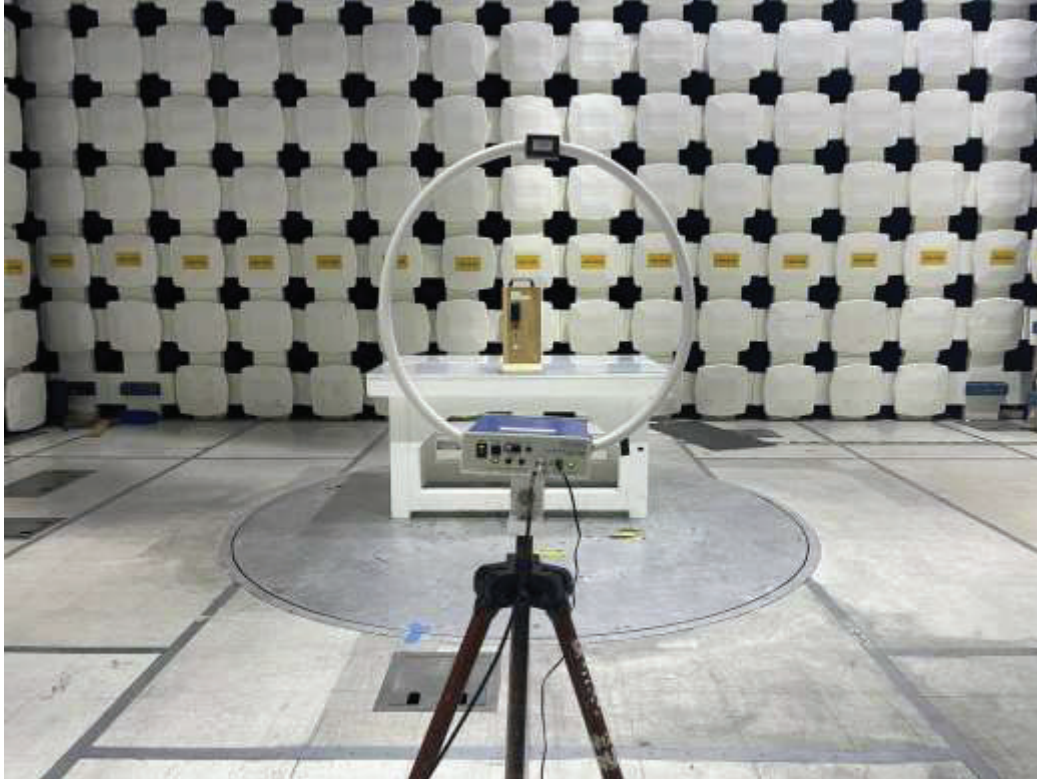
125 kHz and 13.56 MHz RFID (Metal Enclosure) Test Setup, X-axis, RE 9 kHz-30 MHz
