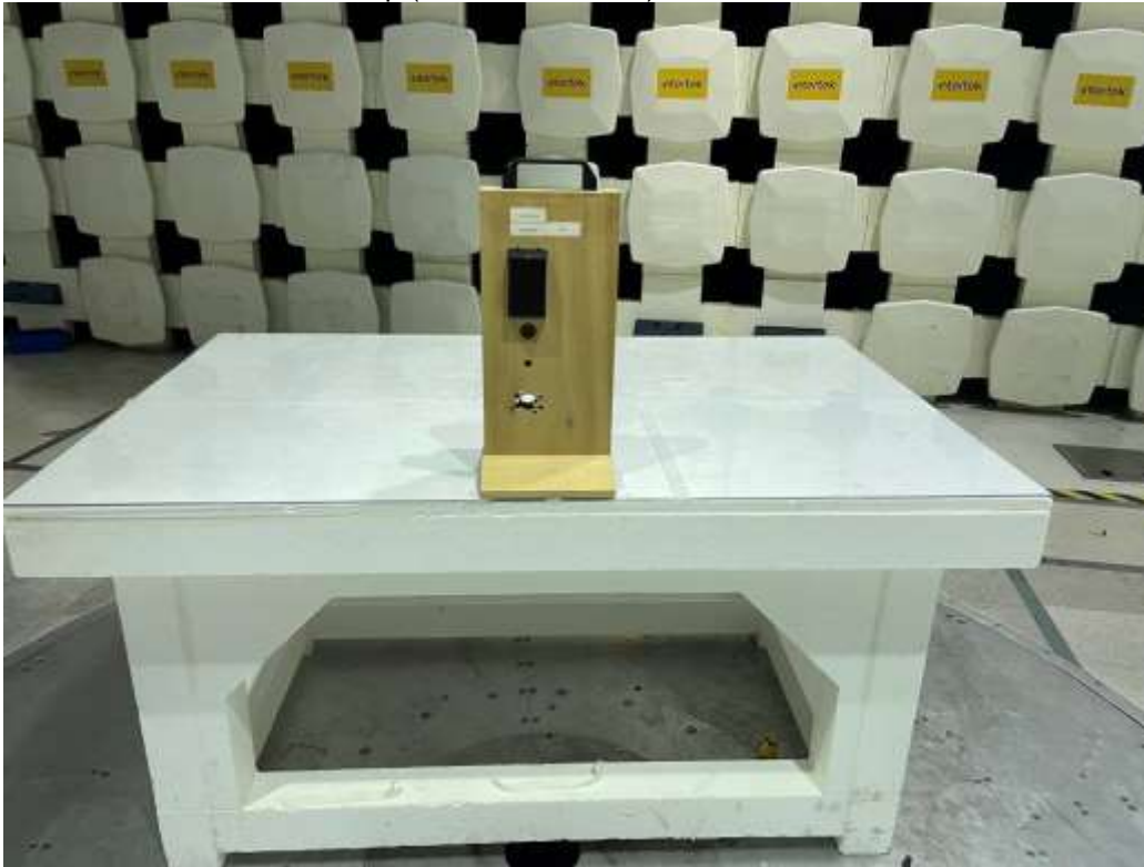
Test Setup (Plastic Enclosure), RE 30-1000 MHz
