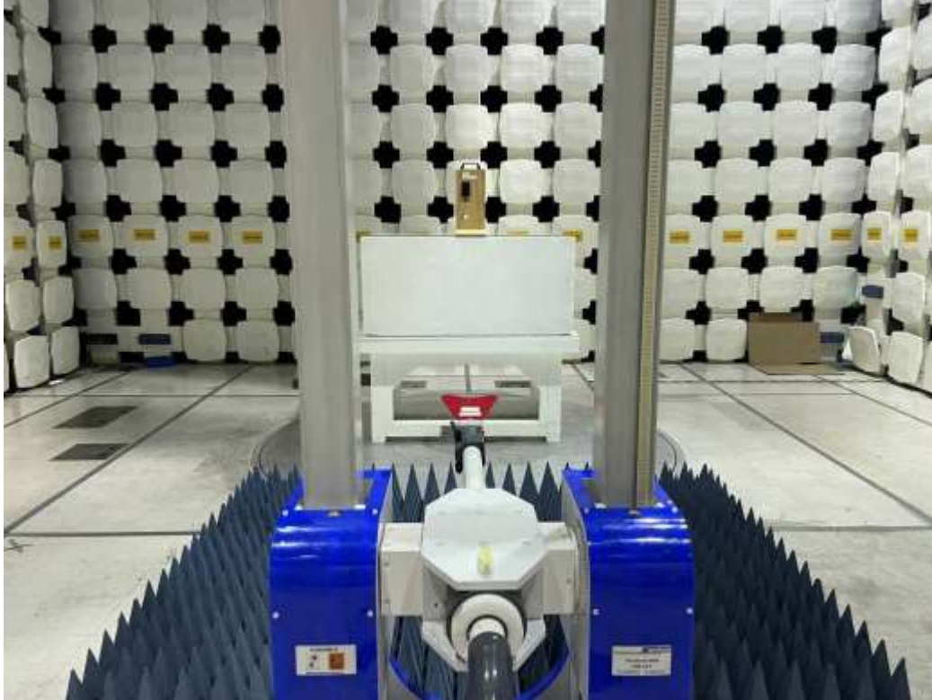
Test Setup (Plastic Enclosure), RE 1-18 GHz
