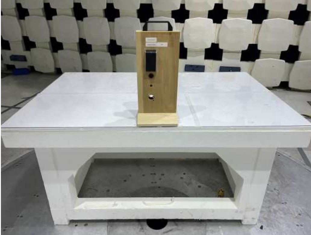
Test Setup (Metal Enclosure), RE 30-1000 MHz
