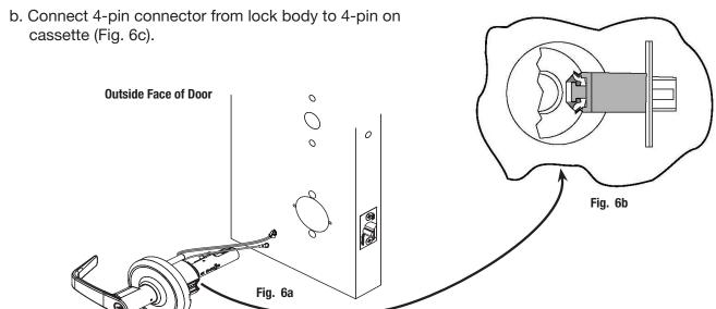
c. Temporarily install top throughbolt to hold chassis in door (Fig. 6c).
