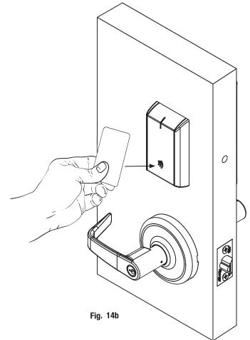
Note: The credential should approach the inscription on the reader as indicated (Fig. 13b) to ensure that the credential is read properly.
