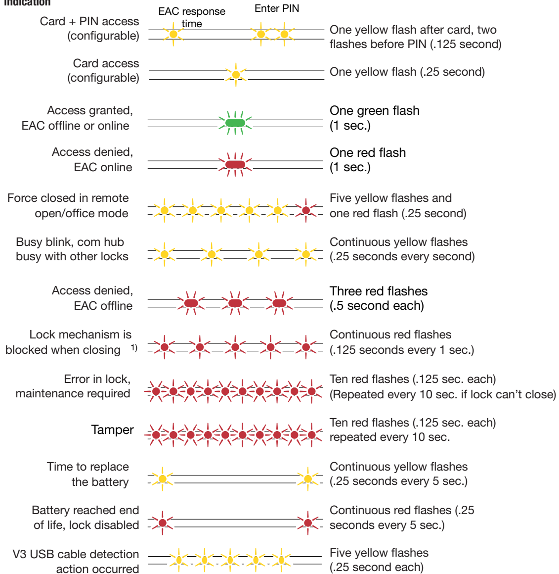
Figure 4. Lock normal operation LED indication
