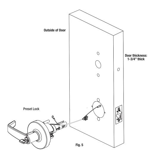
NOTE: Adjusting for a thicker door requires removal of the outside lever, scalp and spacer bushing; see the following sections.
