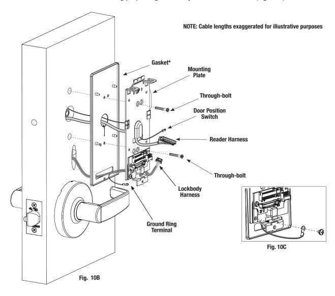
6. Secure ground lug with #6-32 machine screw (Fig. 10C).
