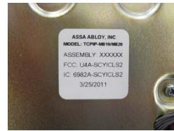
P1-IM/IKM and TCPIP-M819/M820 (FCC Model/ID/IC and Part 15 labels) – Lock Escutcheon
