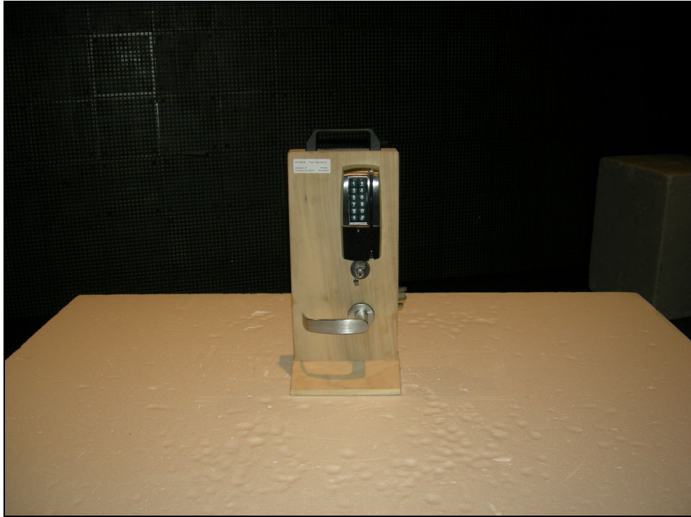
Figure 1: Radiated Emissions – ACCESS700 PWI1-BIMPSK\C ML20700 Battery Powered
