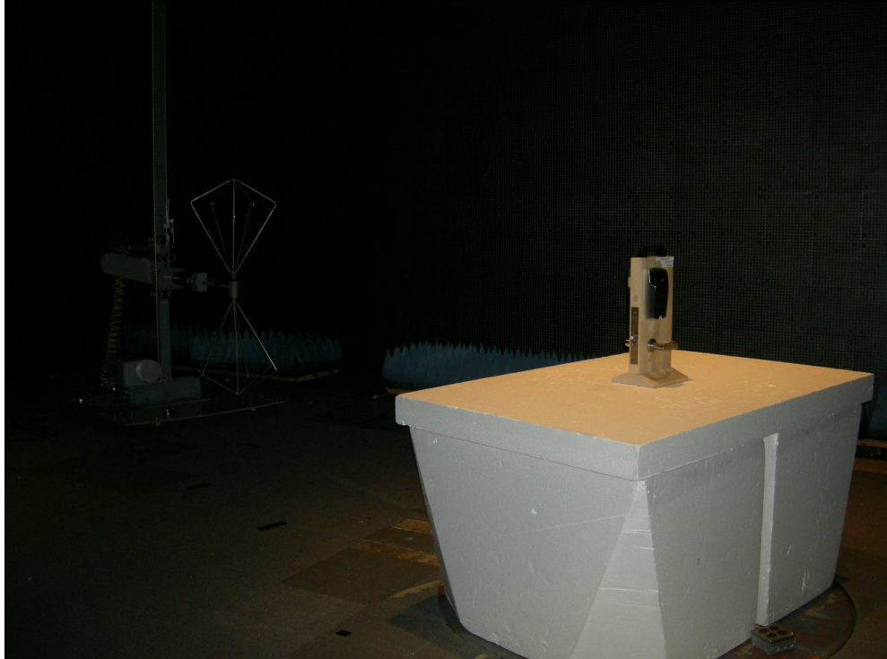
Figure 2: Radiated Emissions – ACCESS700 PWI1-BIMPSK\C ML20700 Battery Powered
