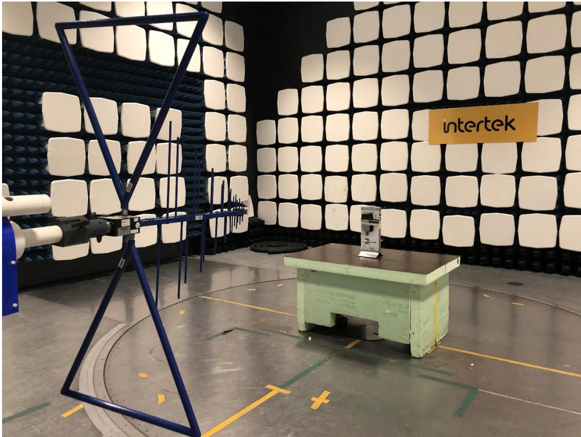
Photo of the test set-up for radiated emission below 1 GHz
