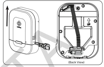
Next, find the connector that comes out of the bottom of the interior escutcheon. Plug the mating connector from the push rail harness into this connector.
