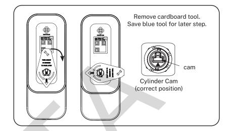
**IMPORTANT:** the blue plastic 'UP' indicator piece may rotate when you turn the cardboard tool. Make sure the blue arrow is always pointing up after you rotate the cardboard tool.
