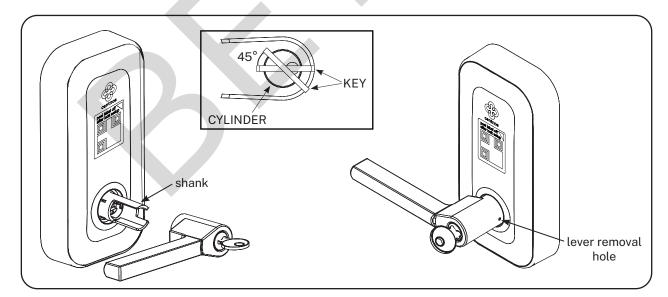
Need to remove the outside lever? Turn the key 45°, press the installation tool into the small hole on the side of the lever. This will depress the lever catch. Then pull the lever and cylinder off the shank.
