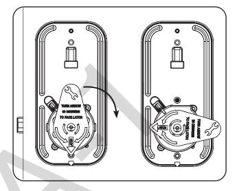
Gently pull the harness through the plate, as you place it against the face of the door, eliminating slack in the harness. You can now secure the mounting plate to your door using two of the #10-32 x 1-1/4" flat head machine screws.
