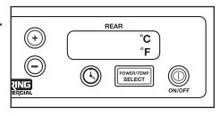
The screen will illuminate and display °C and °F, as seen above. The current setting will blink. Use the + and – buttons to switch to your desired setting. Once your desired setting is blinking, press the POWER/TEMP SELECT button to confirm, and then press the ON/OFF button.
