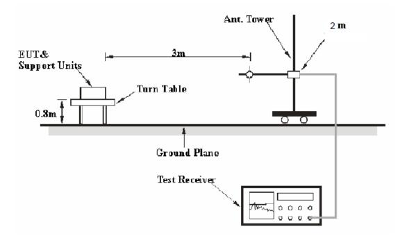
The radiated emission tests were performed in the 3 meters chamber test site, using the setup accordance with the FCC MP - 5.
