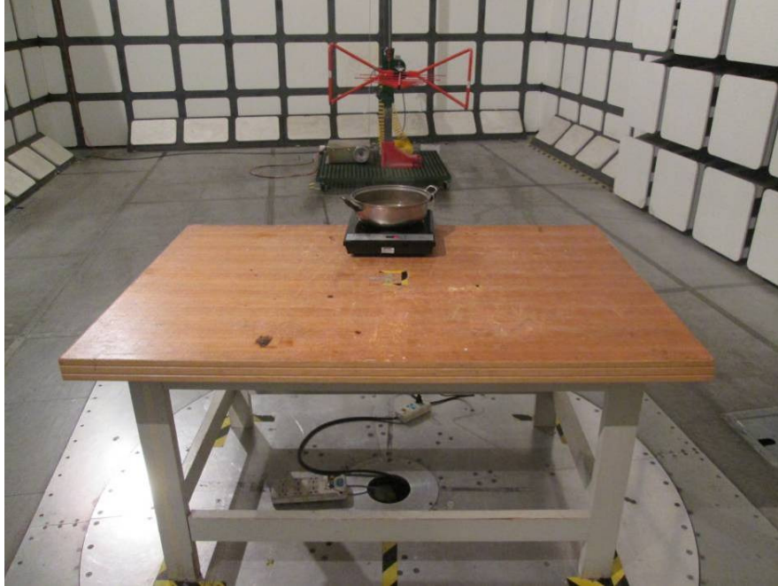
Radiated Emissions - Front View (Above 30MHz)
