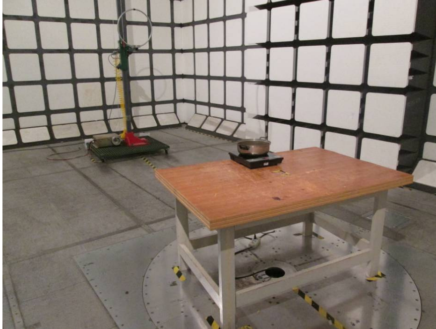
Radiated Emissions - Front View (Below 30MHz)
