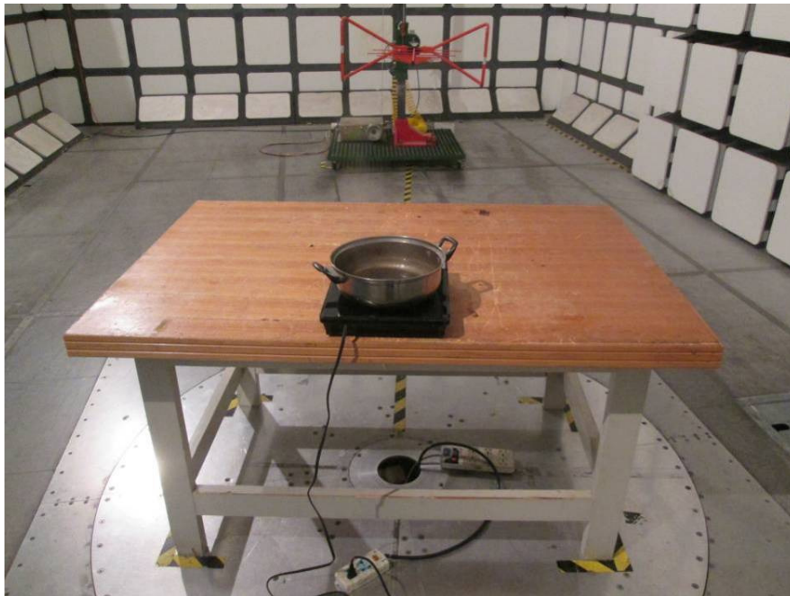
Radiated Emissions - Rear View (Above 30MHz)
