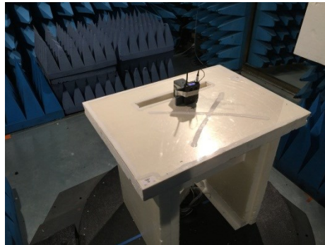
Test setup in anechoic chamber <1GHz
