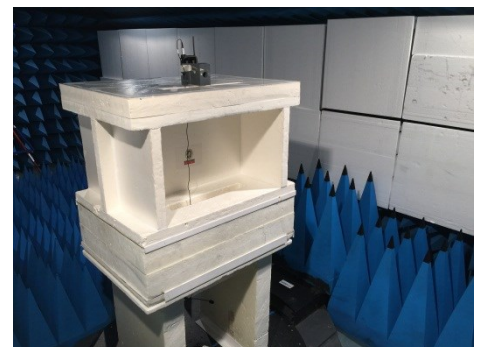
Test setup in anechoic chamber >1GHz (measure performed for the band edge measurement)
