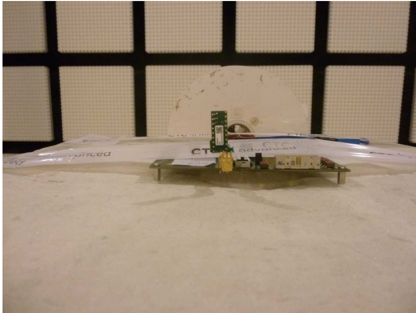
Photo 7: EUT at the anechoic chamber, PCB antenna
