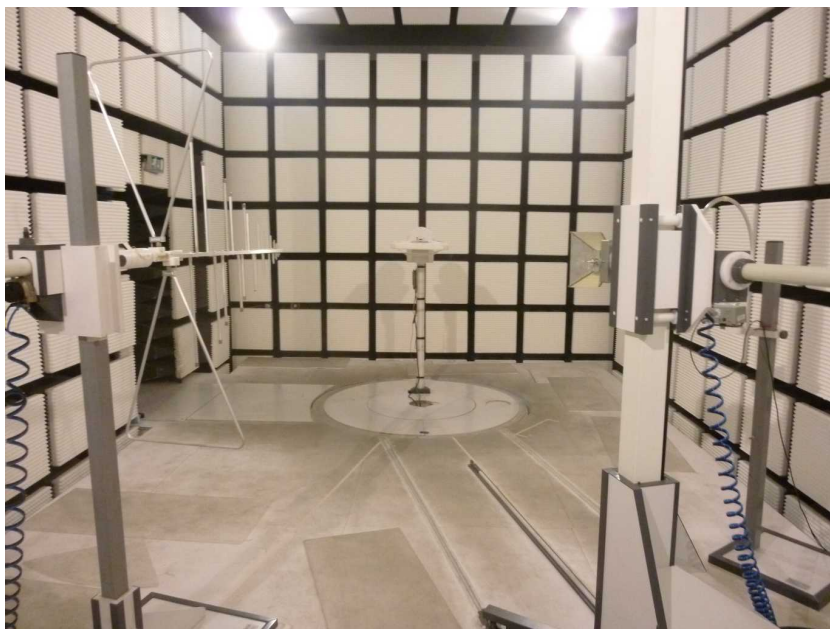
Photo 10: EUT at the anechoic chamber, PCB antenna
