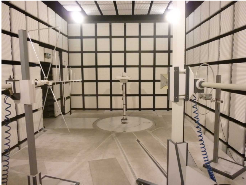
Photo 5: EUT at the anechoic chamber, dipole antenna
