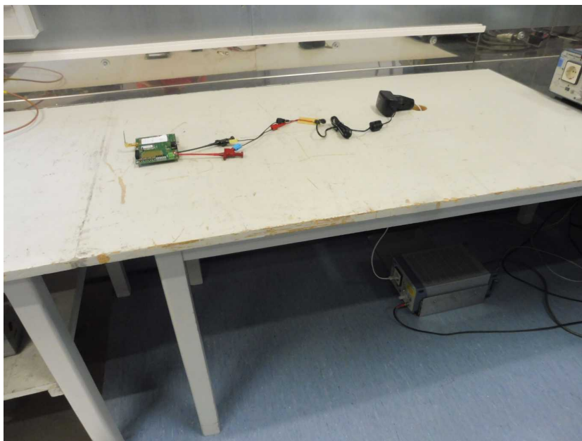
Photo 14: AC conducted emission test setup with PCB antenna
