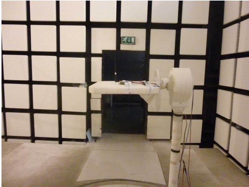
Photo 3: EUT at the anechoic chamber, dipole antenna
