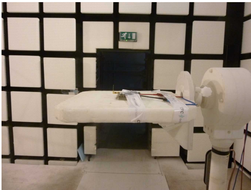
Photo 8: EUT at the anechoic chamber, PCB antenna
