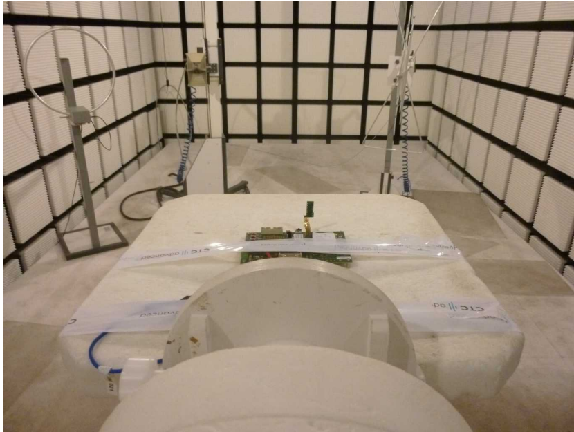
Photo 9: EUT at the anechoic chamber, PCB antenna
