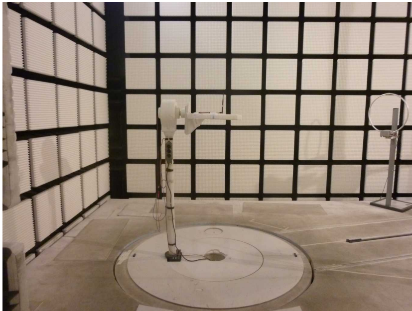
Photo 1: EUT at the anechoic chamber, dipole antenna
