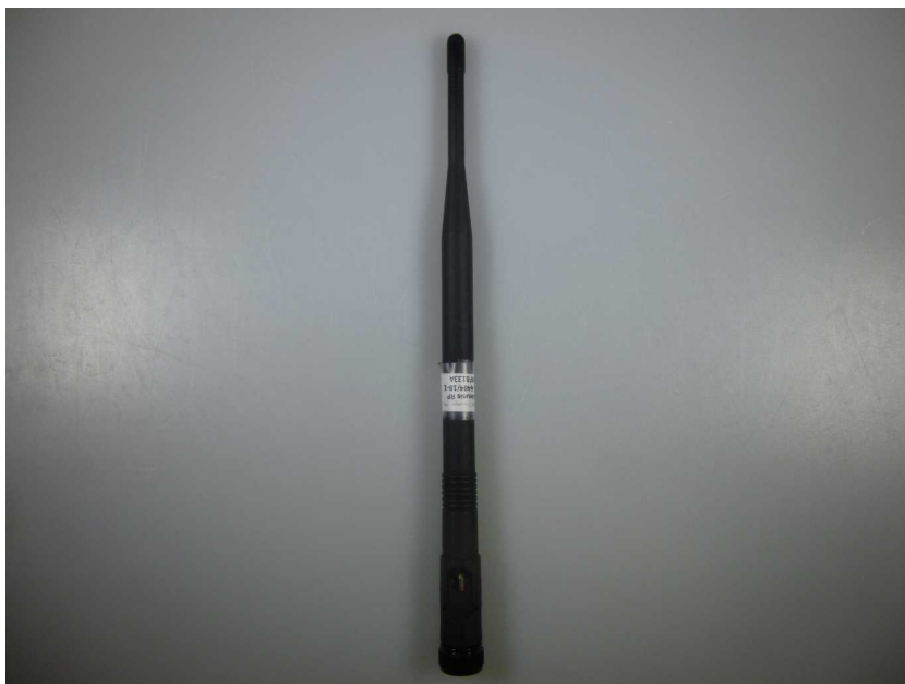
Photo 10: External dipole antenna
