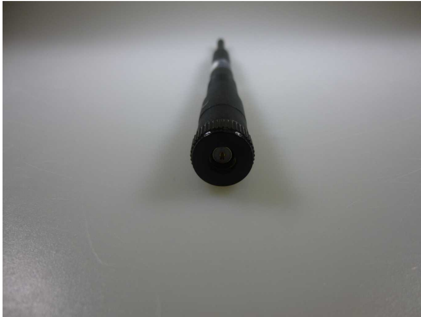
Photo 11: External dipole antenna
