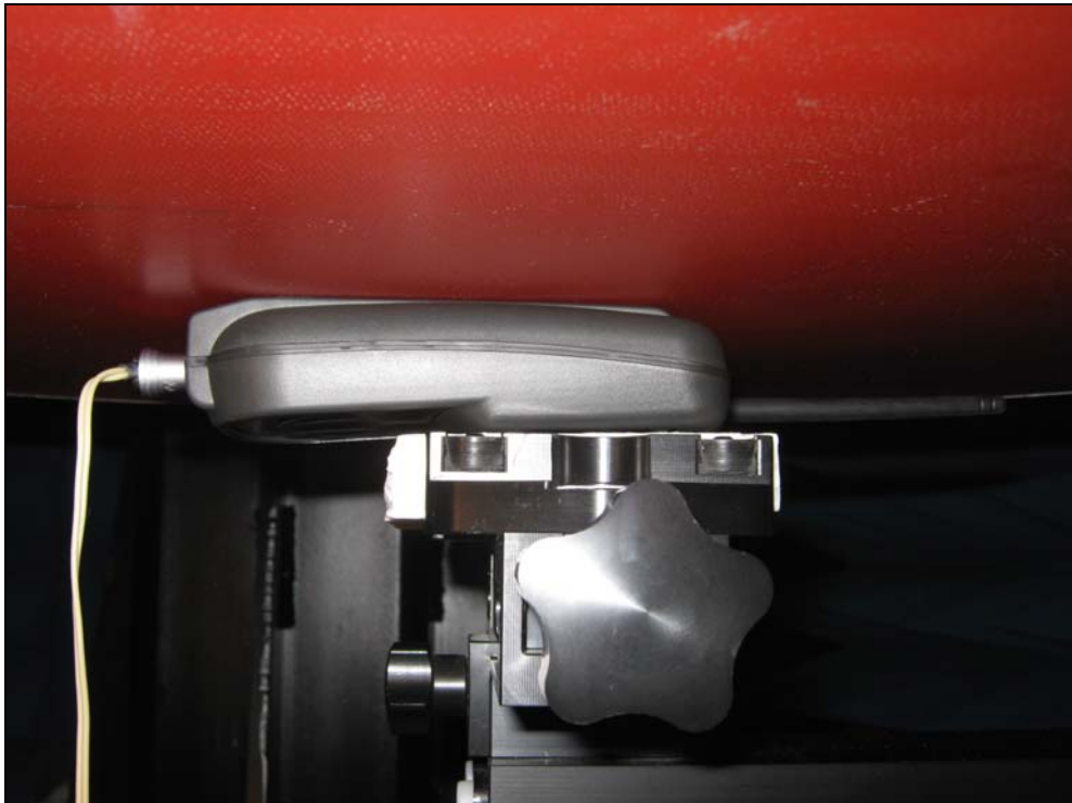
Fig. 4: rear side at 0cm from the phantom with headset + 1130mAh battery
