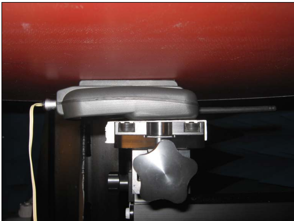
Fig. 6: rear side at 0cm from the phantom with headset + 2260mAh battery
