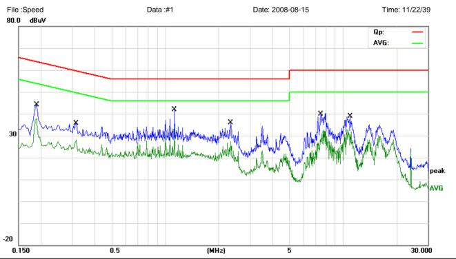
Limit: FCC Part 15B Class B Conduction (QP)
