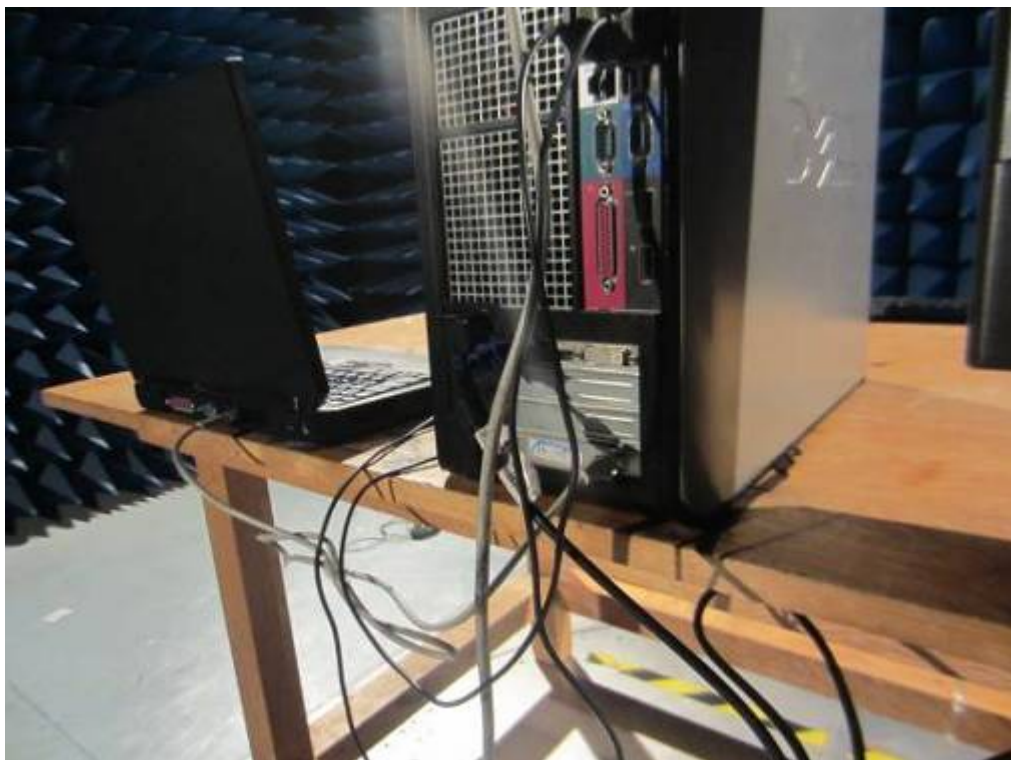
Test photo of radiated emission (30MHz-1000MHz)
