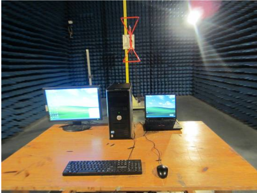
Test photo of radiated emission (30MHz-1000MHz)
