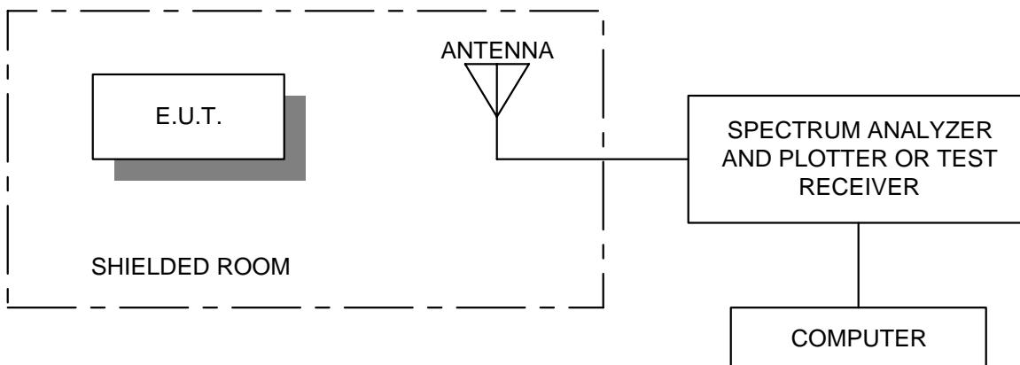
**Test Site For Radiated Emissions**
