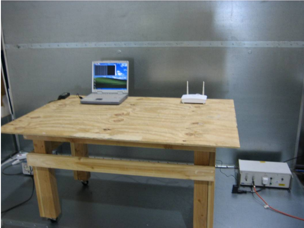
Conducted Emissions Voltage Setup
