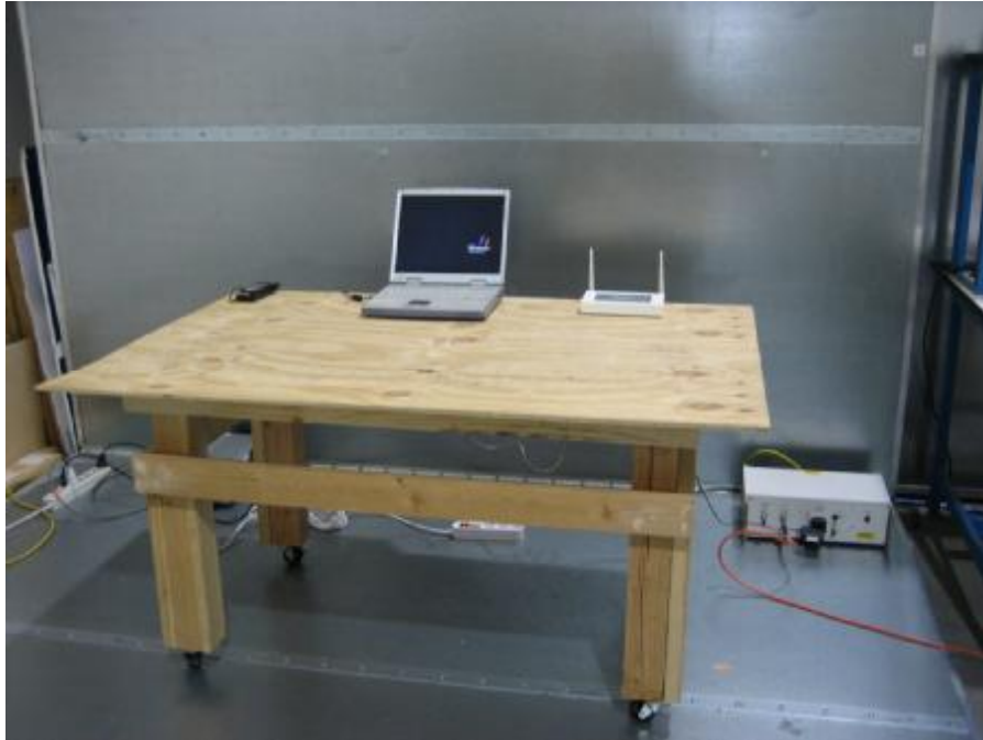
Conducted Emissions Voltage Setup
