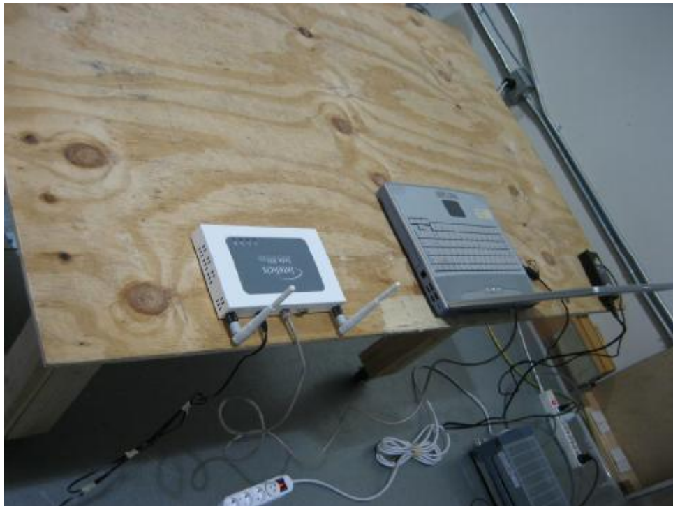
AC Line Conducted Emission Rear View
