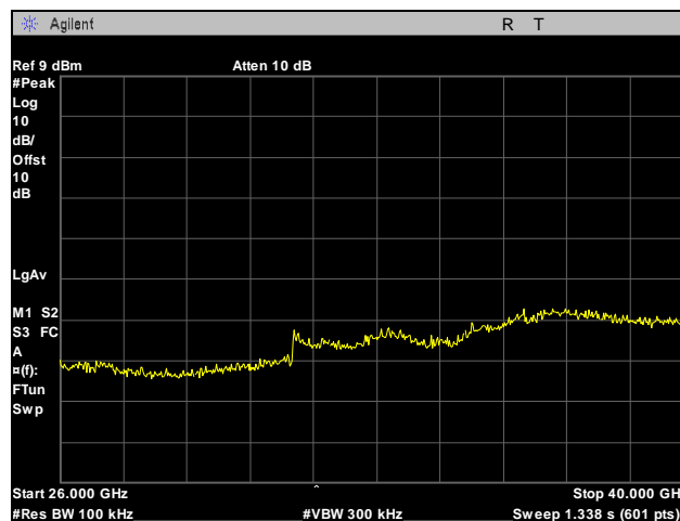
Plot 219. Conducted Spurious Emissions, 802.11n 20 MHz, 5825 MHz, High Channel (26 GHz - 40 GHz)
