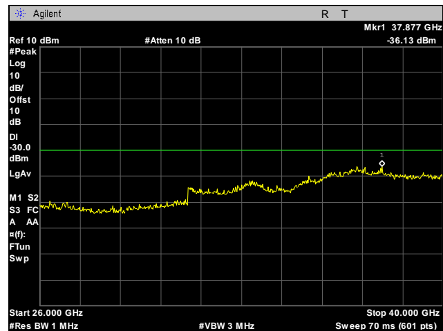
Plot 38. Conducted Spurious Emissions, 802.11a, 4962.5 MHz, 5 MHz, 26 GHz – 40 GHz
