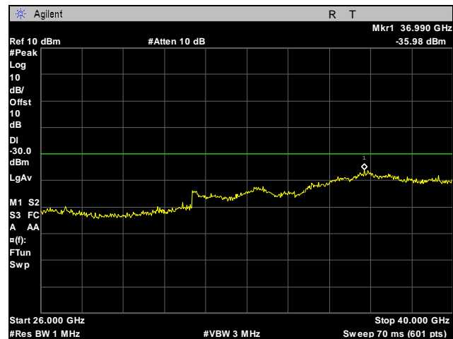
Plot 41. Conducted Spurious Emissions, 802.11a, 4987.5 MHz, 5 MHz, 26 GHz – 40 GHz
