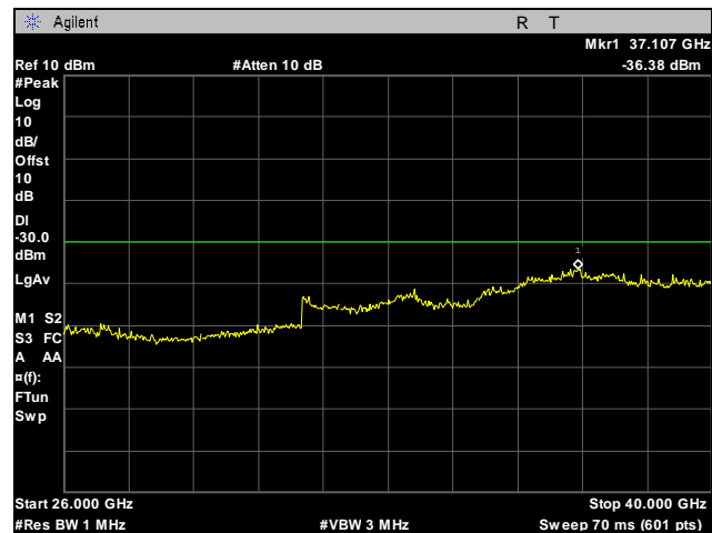
Plot 35. Conducted Spurious Emissions, 802.11a, 4942.5 MHz, 5 MHz, 26 GHz – 40 GHz
