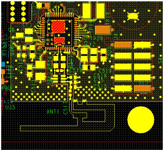
Fig 1. RF circuitry layout showing with ground plan in layout design.
