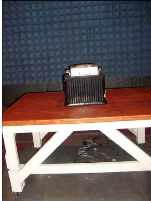
Photograph 1. Radiated Emission Spurious Test Setup
