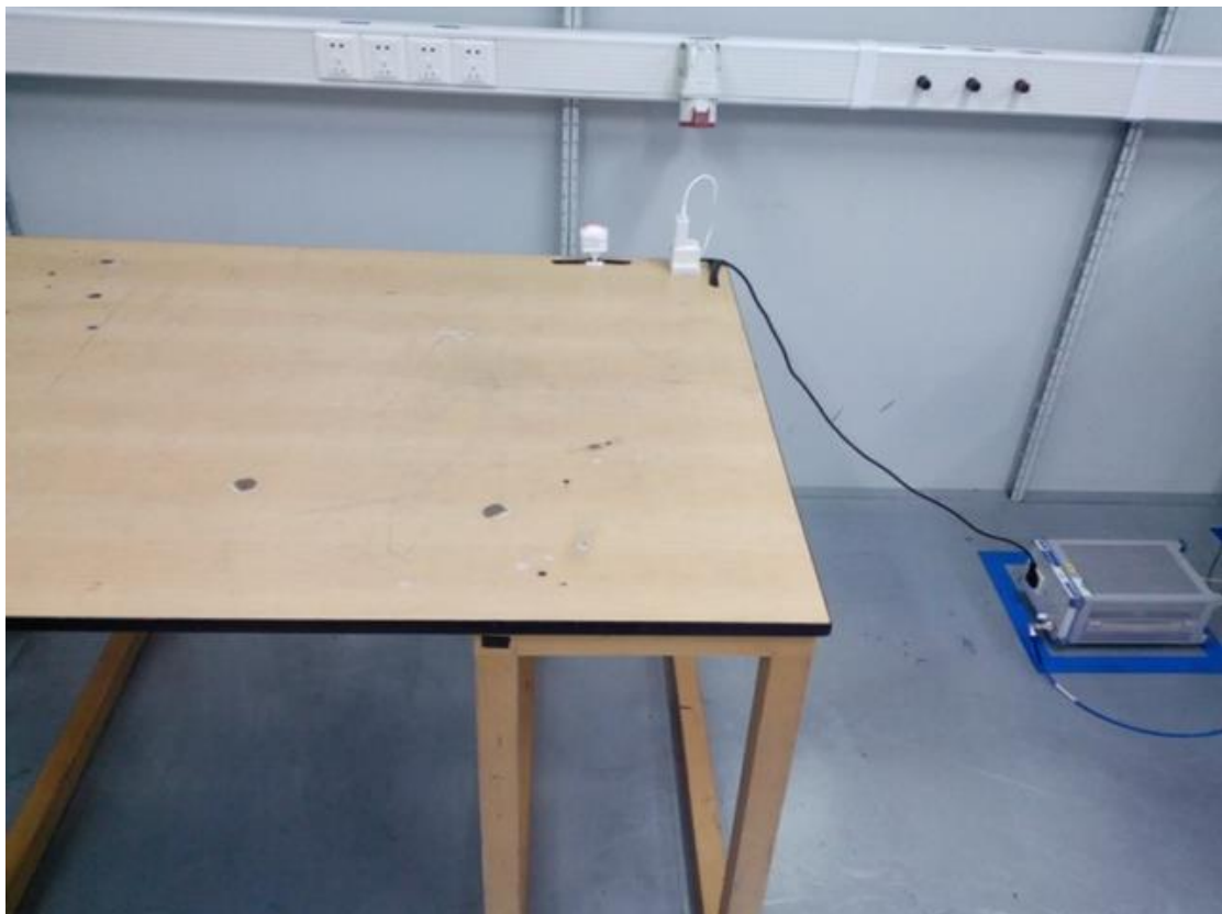
AC Conducted Emission Test Setup -Front
