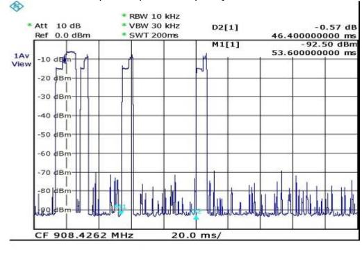
The device with a pulse-repetition frequency less than 50 ms.
