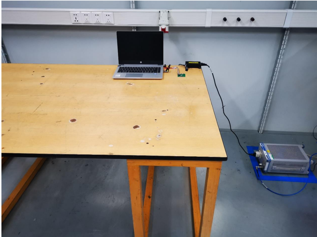
AC Conducted Emission Test Setup -Front
