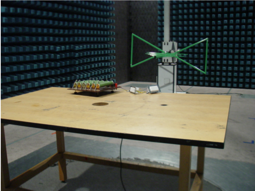
Photo 4 Radiated Emission Test
