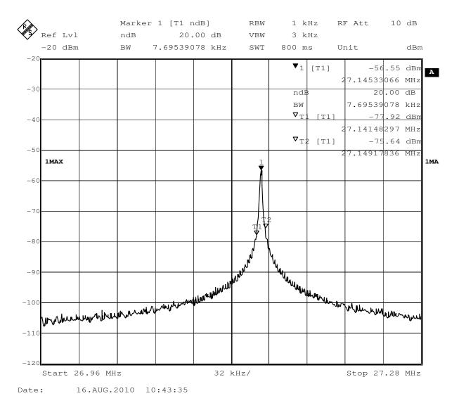
20dB bandwidth lower frequency: 27.14148297MHz 20dB bandwidth upper frequency: 27.14917836MHz The results: The unit does meet the FCC requirements
