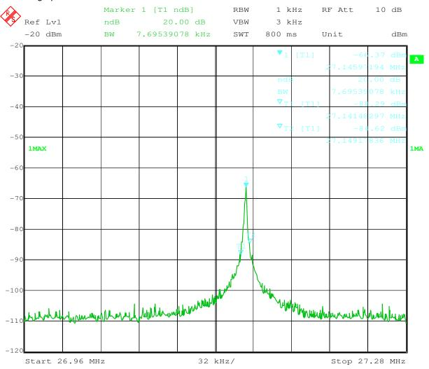
20dB bandwidth lower frequency: 27.14148297MHz 20dB bandwidth upper frequency: 27.14917836MHz
