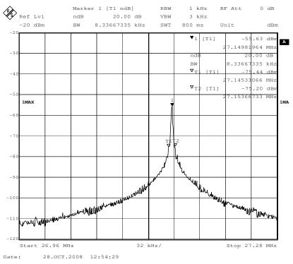
20dB bandwidth lower frequency : 27.14533066MHz 20dB bandwidth upper frequency : 27.15366733MHz
