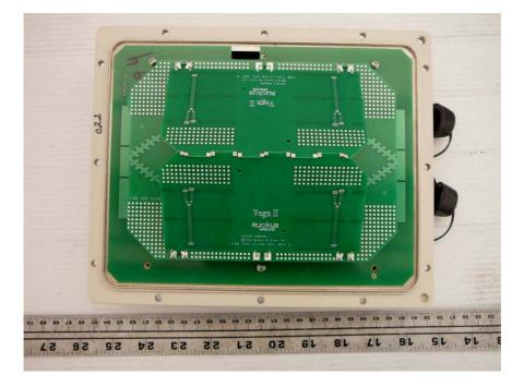
16.10 EUT- 8 dBi Internal Antenna Board Top View
