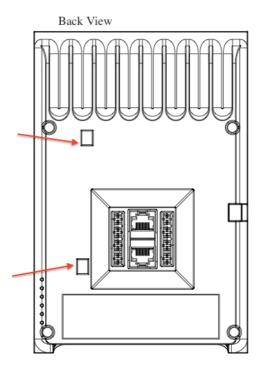
A of the bracket goes to holes on the back of the AP.
