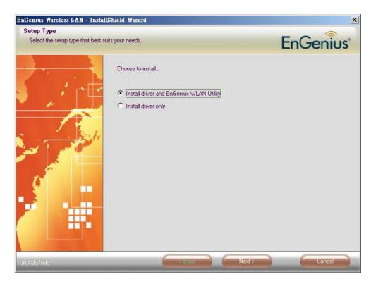
3. Once the setup begins you will see the **InstallShield Wizard**. Select **Install driver and EnGenius WLAN Utility** and then click on the **Next>** button.
